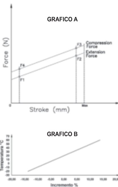
A gas spring has a progressive movement and follows a trend which is generally expressed in the following graph:
